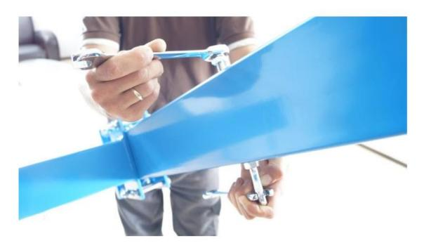
13. The next stage is attaching the vertical beam with the suspension base beam. Align the hole son the vertical beam onto the base beam holes.
