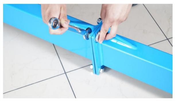
9. Before attaching all the suspension beams together, it is recommended to install the extension beams or a clamp on the horizontal beam.
